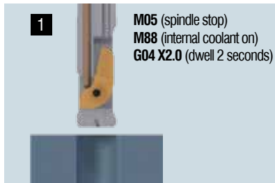
Minimum internal coolant pressure: 280 PSI (19.3 BAR)
